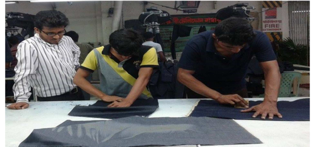
Figure 2. Hand Sand Process.
